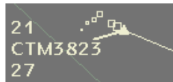
Fig. 1. The ODS comet of an evolving aircraft, the image exhibits direction and acceleration changes
